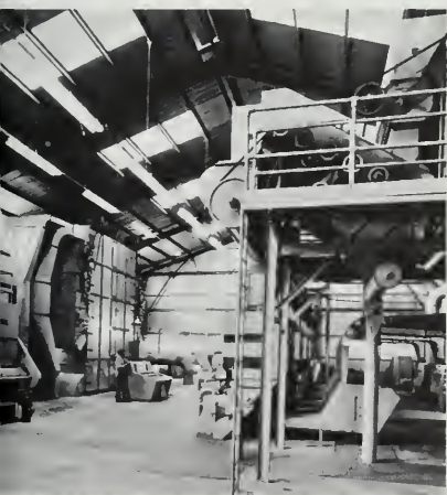
A modern cotton gin with elaborate drying and cleaning equipment for handling machine-harvested cotton represents an investment of about 250 thousand dollars.
